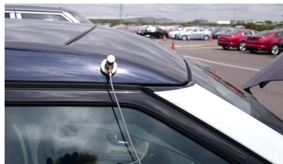
Figure 2 (b): Close ups of the measurement response position above upper A-pillar.
